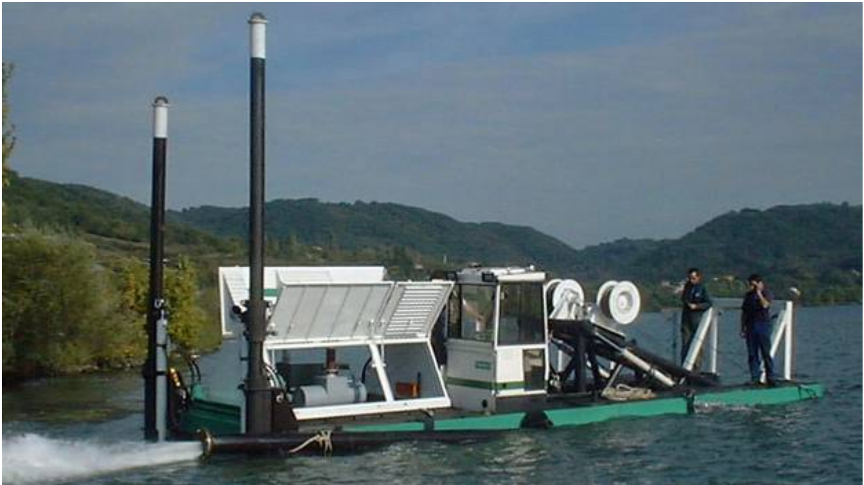
Figure 6: Hydraulic cutter dredge with 8-inch diameter discharge pipe – 2 hydraulic spuds – 200 Hp diesel engine with clear water pumping capacity of 600-900 CY per hour – 44 feet in length with maximum draft of 2.5 feet.
