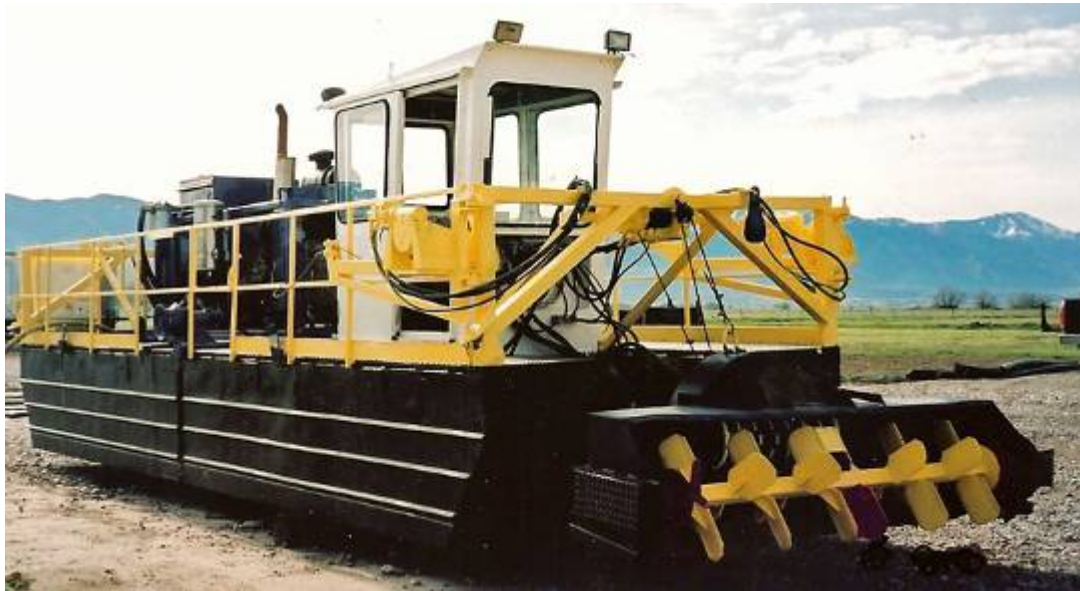
Figure 5: Horizontal auger hydraulic dredge with cable winch – 174 Hp diesel engine with 10-inch diameter discharge pipe.
