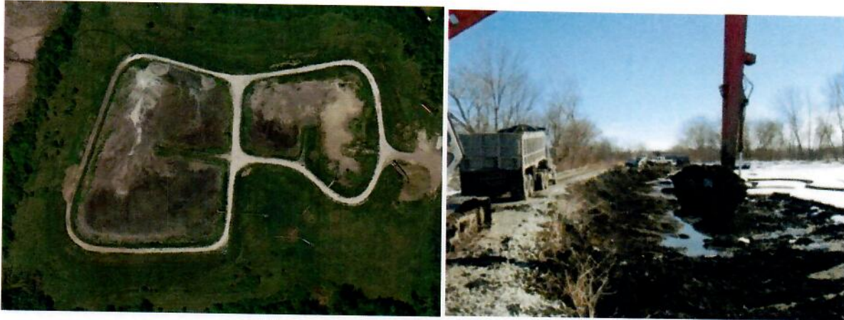
Figure B14: Sediment dewatering facility (SDF) allows for permanent sediment and dewatering. Once sediment is dewatered it can be harvested for reuse. Photos courtesy of Google Earth and Fox Waterway Agency respectively.
